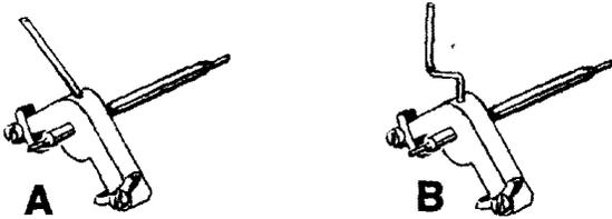
Most anchor pins are threaded and screwed into the pallet base but I have seen these pins soldered. Just be sure how the anchor pin is secured and if it's hardened, BEFORE you make any adjustments and have a look on pages 42 & 43 in the 10<sup>th</sup> edition, for most of the variations on anchors and escape wheels. If you do bent the anchor pin then repolish it and I use 4/0 steel wool followed by 4/0 emery paper.
