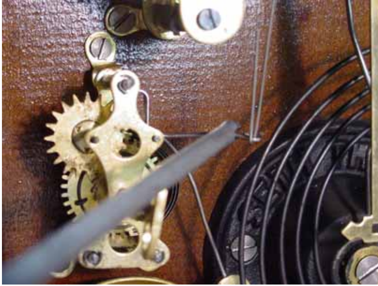
Adjusting the release arm for the proper start and stop of the alarm.
