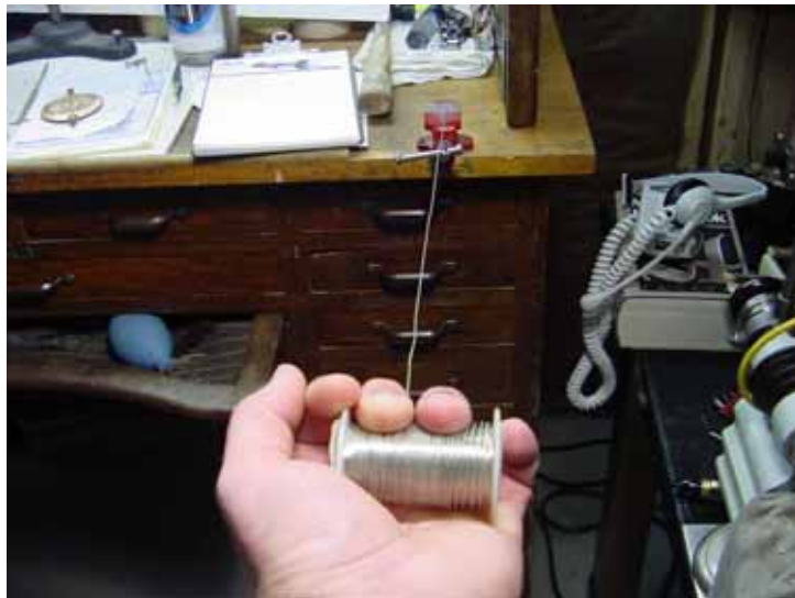
Stretching soft wire to make a new alarm release wire.
