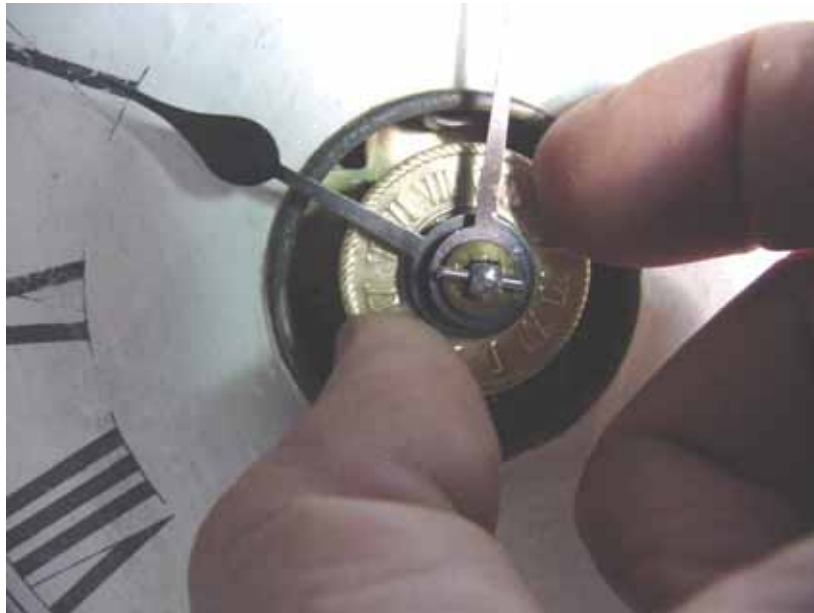
Setting the alarm to go off at 5:30. Note the position of the set disk under the hour hand.
