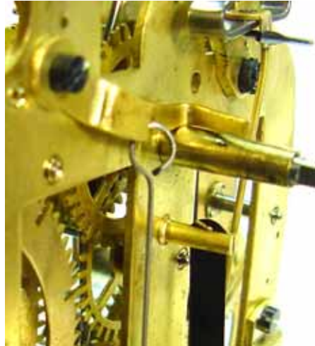
New wire, looped and attached to the alarm release lever.
