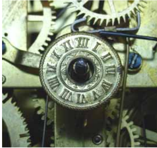
Proper position of the alarm set disk at the point of release.
