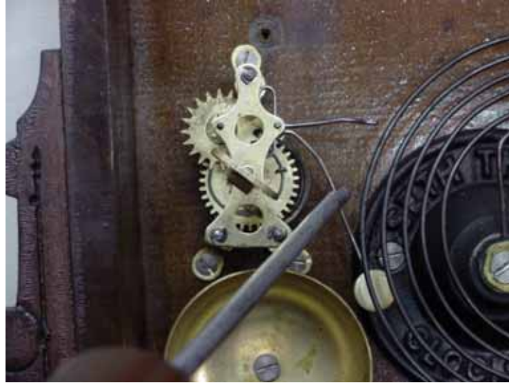
Adjusting the hammer arm to properly strike the bell without binding the alarm anchor.
