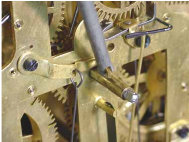
Adjusting the alarm release lever to obtain the correct release point.
