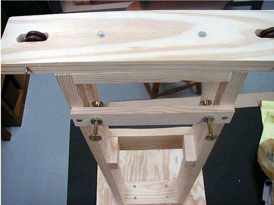
8. **Back Brace – Made from a scrap piece of wood 1 1/4 inches high x 8 1/4 inches wide – approximately 3/8 inches thick.**
