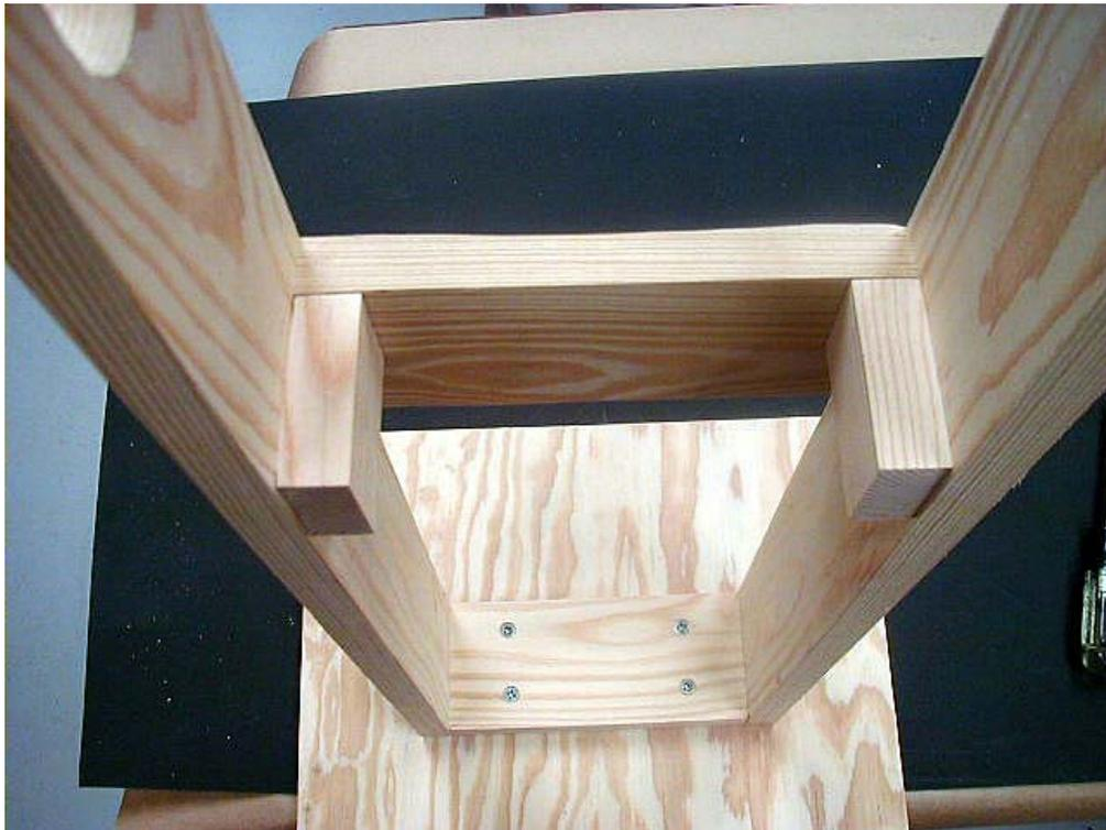
**Mount flush with top of front support with two # 10 x 1 1/4 inch wood screws (Before installing second screw, place test stand on a level surface and check to make sure side supports are level. Adjust as needed).**
