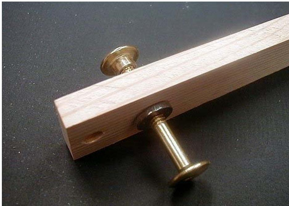
**Tap in the insert nuts and then install the connecting bolts and caps. Use Loctite to secure nut to bolt. (Cap nut is on inside of the back brace board.)**
