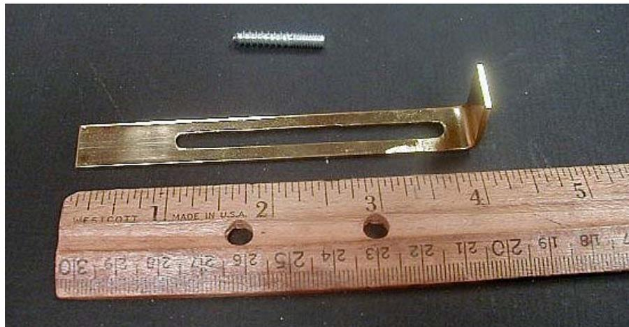
**Drill a 3/16<sup>th</sup> inch hole at each end of the marked slot. Scribe parallel lines to join the outer edges of the two drilled holes. Using a jeweler's saw, cut along the scribed lines to complete the slot. The slot should be about 3/16<sup>th</sup> of an inch wide and should clear the threaded ends of an 8-32 hanger bolt. File the slot edges smooth. Polish and lacquer the brass to prevent tarnishing.**
