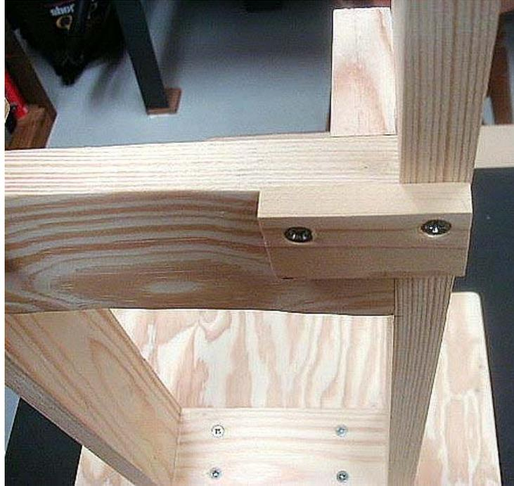
**Install with two - # 8 x 1 inch wood screws such that a bottom lip is formed of approximately 1/8 inch to 3/16 inch.**
