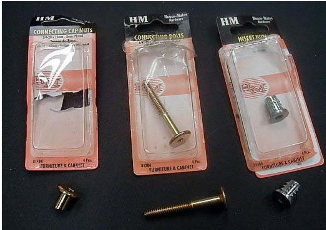
**The drill point for the insert nuts are at 1 1/4 inch from each end of the back brace. Drill a 11/32 inch hole at each drill point. (Part of the insert nut is ground off to make it flush with the thickness of the back brace. Similarly, about 1/4 inch of the connecting cap nuts is ground off to allow more travel room for the bolt.)**
