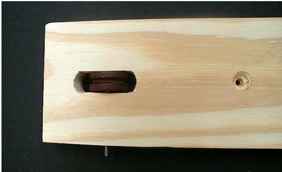
The pulleys will need to be opened up a bit with a 1/8 inch drill. Make sure the pulleys spin freely on the arbors before installation. Insert each arbor and slip on the pulleys. Tap the arbors to seat them in place. I recommend leaving about 1/2 inch of the arbor remaining in case it ever needs to be removed.
