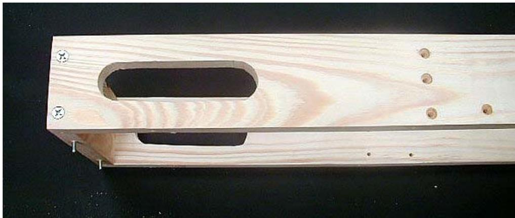
**Note:** The slot shown in the accompanying photo is too short – the dimensions have been revised as shown above.
