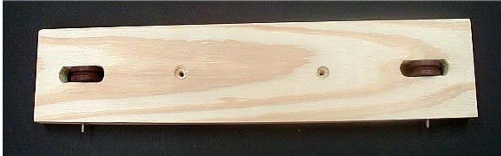
The arbors for the pulleys are made from 1/8 inch steel rod (Lowe's). Grind a point on one end. From the back side of the top piece, drill a 1/8 inch hole for the arbor in the center of each of the two pulley openings. Make sure that the drill is level in order to keep the hole centered on the opposite side of the opening. Drill through about 1/2 inch on the opposite side.
