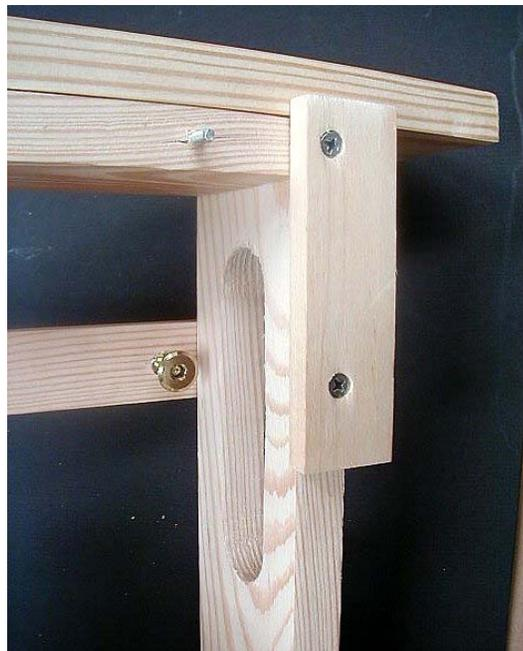
**Mount the braces with 2 - # 8 x 1 inch wood screws on the left and right sides of the frame such that a lip is formed of approximately 1/8 inch to 3/16 inch.**
